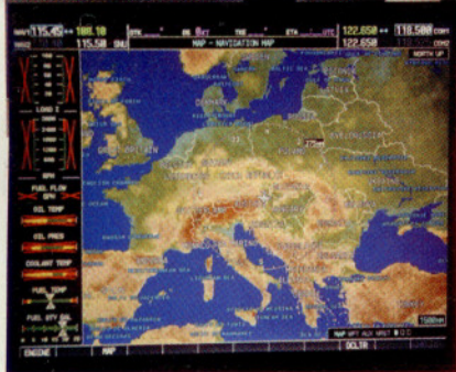
The avionics package features a two-display Garmin G1000. Its multifunction display can be zoomed in or out (left) to show a massive moving map. Diamond's Austrian factory is in the dead center of the screen. For now, a Bendix/King KAP 140 serves as autopilot; a Garmin unit will soon replace it.
